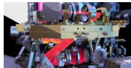
Light travels through the Tropomi instrument thanks to freeform optics. Purple represents UV, red is near infrared and yellow is visible light.
