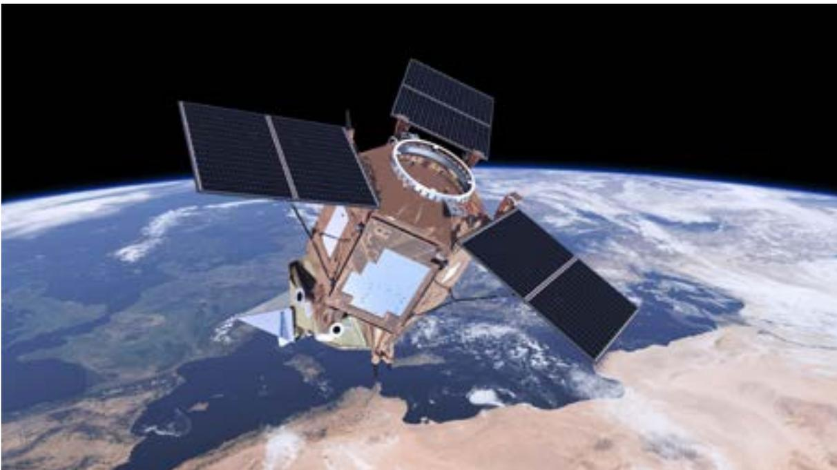
*Sentinel-5P with the Tropomi instrument on board for air quality monitoring. (© ESA-ATG medialab)*
