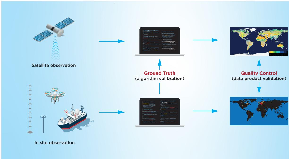
*The important role of in situ data and calibration/validation (cal/val) in the processing and application of EO data.*
